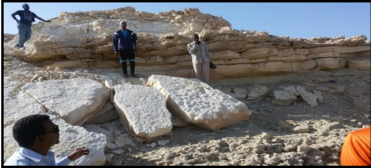
Plate 4: The Sliding of layers of the bedded calcareous calystone lies below the dolomitic limestone.
